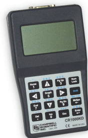
One CR1000KD can be carried from station to station in a CR1000 network.
